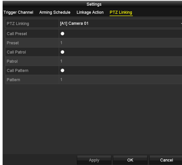
Figure 8-9 Set PTZ Linking of Alarm Input
