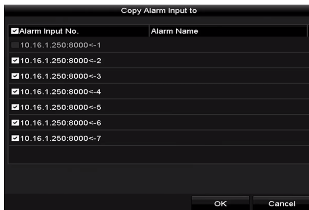
Figure 5-20 Copy Alarm Input
